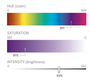
Using the color bars, simply select the desired hue (color), saturation level and intensity (brightness) for any light or group of lights in the Luxor ZDC system. You can save custom colors for easy access.
